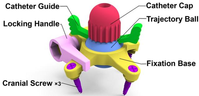
**Fig. 1** Fixation device main parts assembly
