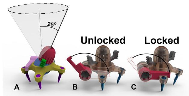
**Fig. 2** Fixation device mechanism schematics. **A:** Trajectory ball 2 angular degrees of freedom (DOF). **B:** Ball mechanism at unlocked state. **C:** Ball mechanism at locked state
