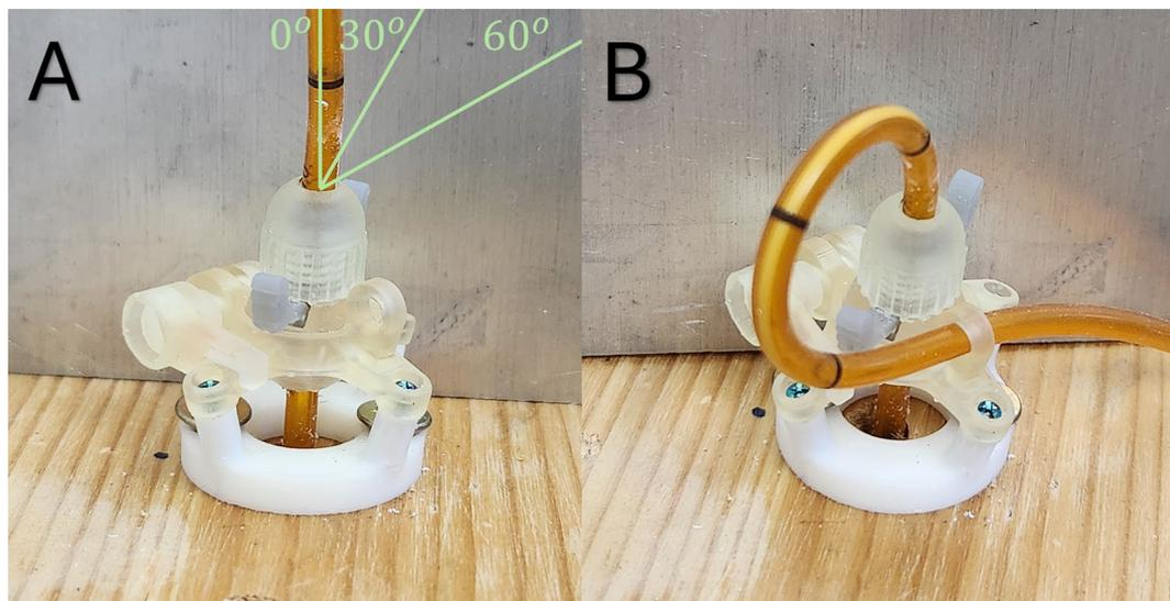
**Fig. 5** Fixation device used without (A) and with (B) a safety loop. Free catheter pull angles are marked in A
