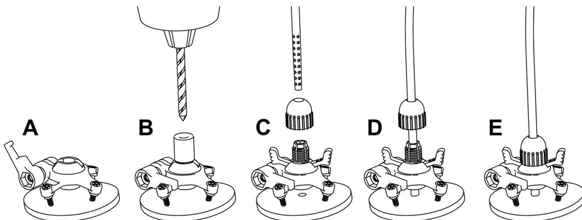
**Fig. 4** Fixation Procedure Steps. **A:** the fixation device is positioned, and the insertion trajectory is determined. **B:** the trajectory ball is locked in place, the drill guide inserted, and a drill is used in the desired trajectory. **C:** the catheter guide is inserted. **D-E:** the catheter is inserted to the desired depth and the cap is locked to the catheter guide
